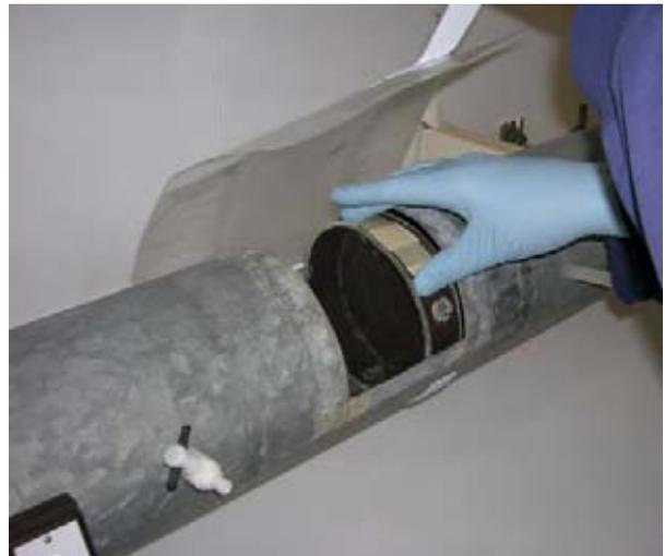
Figure A3.4. Sealed cage being positioned in wind tunnel (courtesy of Dr Jane Bonds, Florida A&M University, Panama City, Florida, USA)
