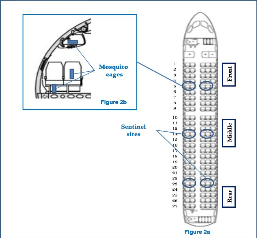
Figure 2. Layout of mosquito cages in a single-aisle aircraft
